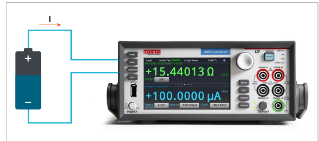
Use a Keithley 2450 or 2460 Series SMU with a model generating test script to discharge batteries and create battery models for the 2281S-20-6 Battery Simulator.
